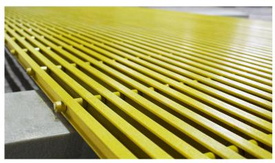
**Pultruded gratings** are prefabricated structures made of fiberglass reinforced plastic profiles (GFRP). The bearing profiles of the I-shaped section have geometric dimensions of 25x15 mm (Type No. 1), 38x15mm (Type No. 2), or 50x25 mm (Type No. 3). They are connected with the help of GFRP rods that have the center-to-center distance of 200 mm.
